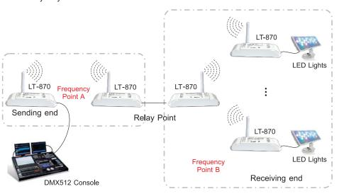
5.3 Extend the communication distance by boost antenna:
